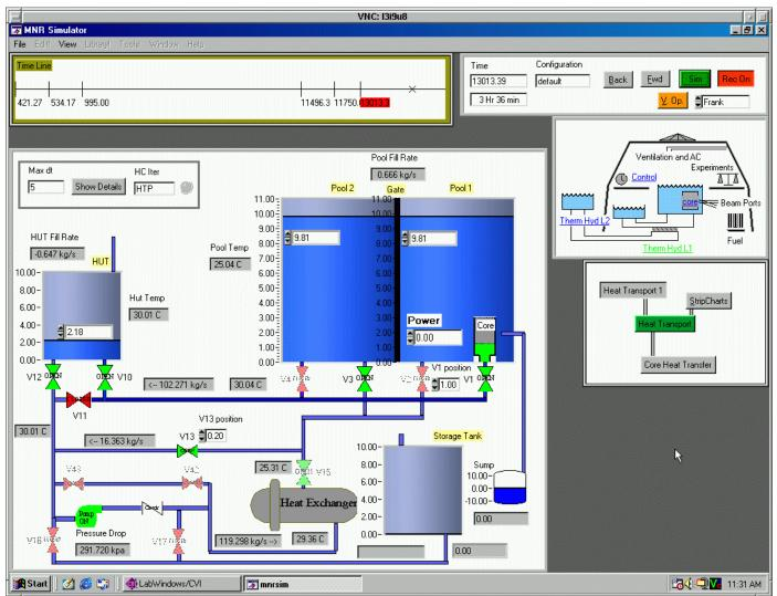
Interface combines flow, temperature distributions, and valve controls.
