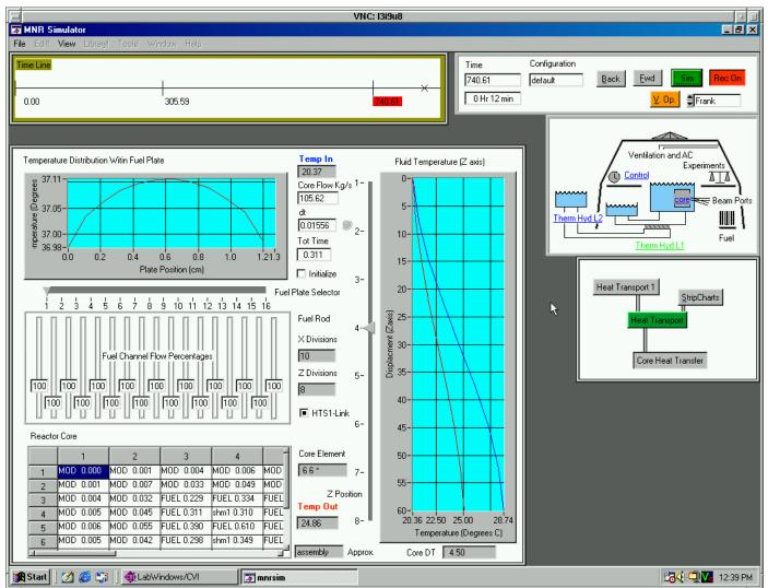
Flux shape is used to compute transient temperatures in fuel rods.
