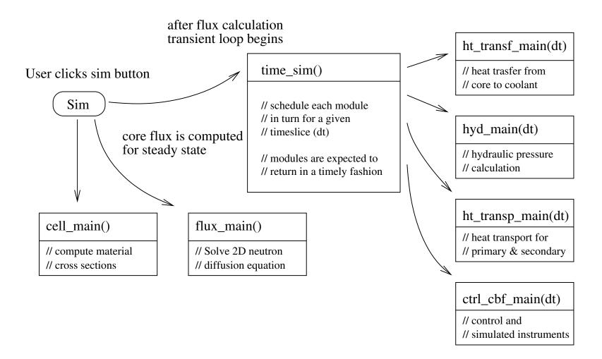
MNRSIM is written in C and compiles under LabWindows. 12,000 lines of code define 20 modules, 7 for physics, 9 for user interface, 4 are general purpose.
