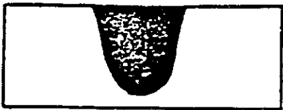
DC Electrode negative -- deep penetration narrow weld
