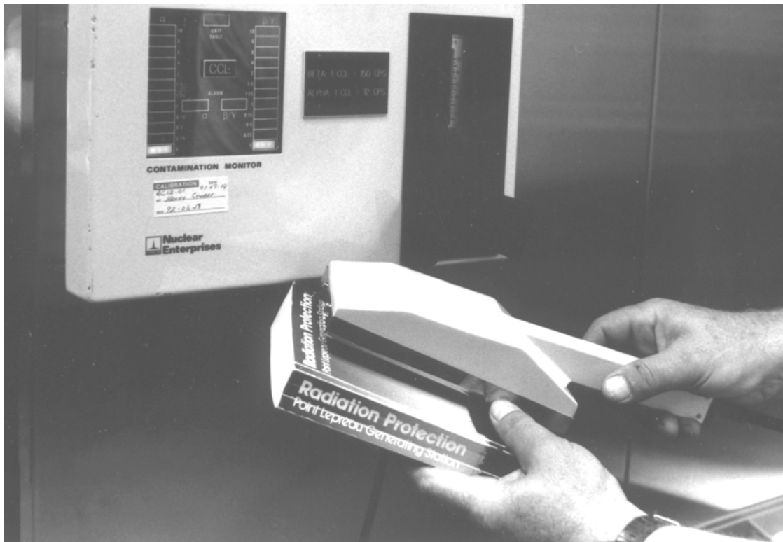
Fig. 9.4. Using the \alpha/\beta,\gamma Contamination Monitor to Check a Book
